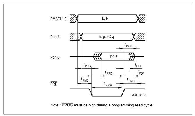
Figure 11-9 Version Byte Read Timing
