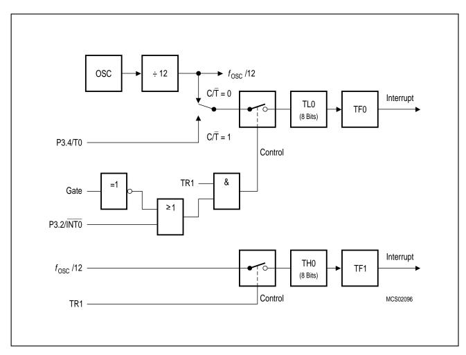
Figure 6-15 Timer/Counter 0, Mode 3: Two 8-Bit Timers/Counters
