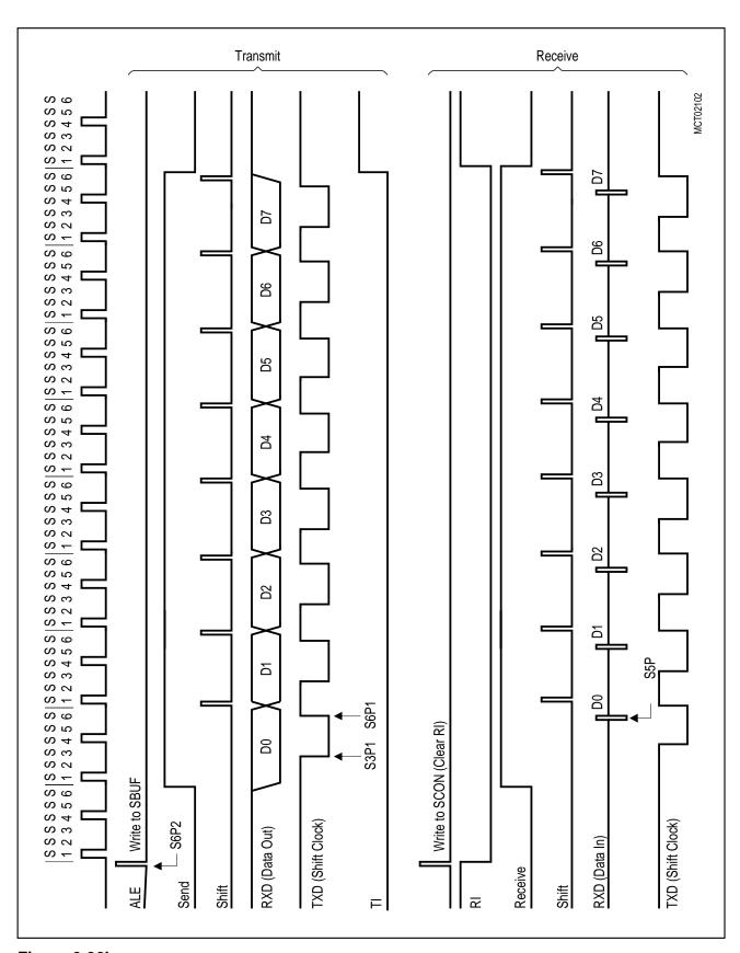
Figure 6-36b Serial Interface, Mode 0, Timing Diagram
