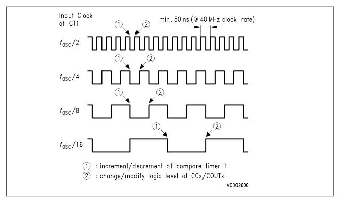
Figure 6-20 CAPCOM Unit Clocking Scheme
