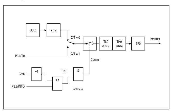
Figure 6-13 Timer/Counter 0, Mode 1: 16-Bit Timer/Counter
