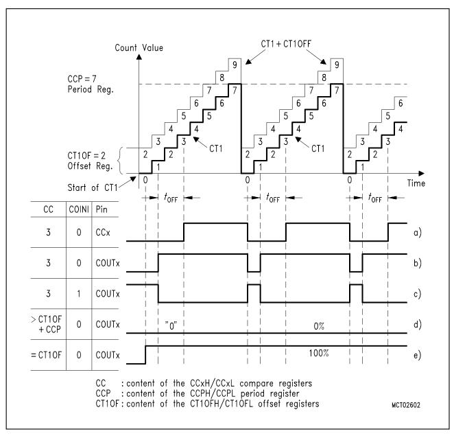
Figure 6-22 Compare Timer 1 with Offset not equal 0 - Mode 0
