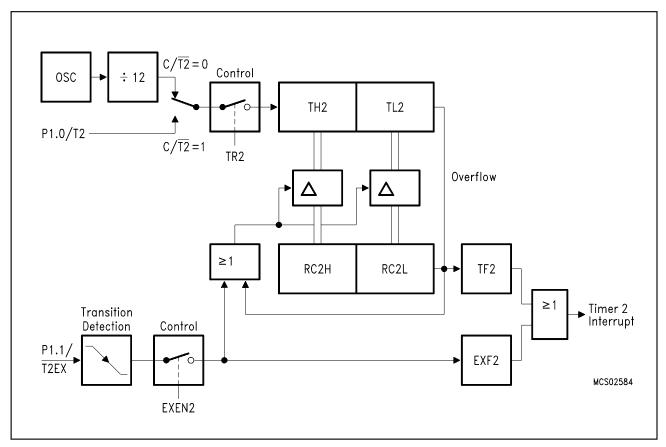
Figure 6-16 Timer 2 Auto-Reload Mode (DCEN = 0)
