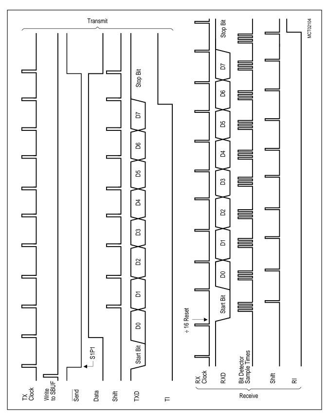
Figure 6-37b Serial Interface, Mode 1, Timing Diagram
