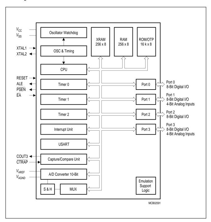
Figure 2-1 Block Diagram of the C504
