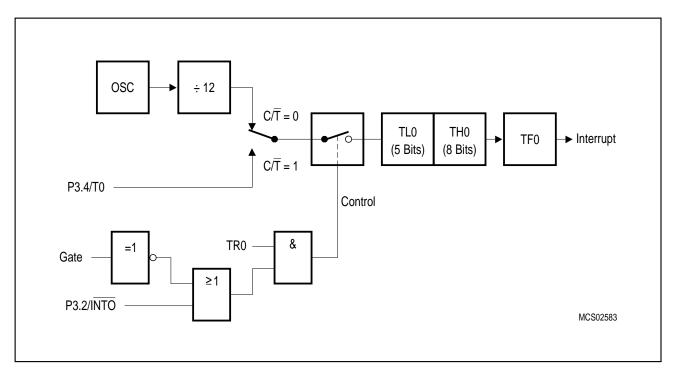
Figure 6-12 Timer/Counter 0, Mode 0: 13-Bit Timer/Counter
