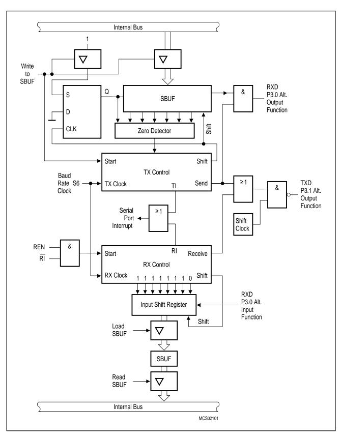
Figure 6-36a Serial Interface, Mode 0, Functional Diagram
