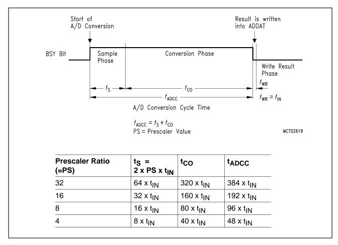
Figure 6-41 A/D Conversion Timing
