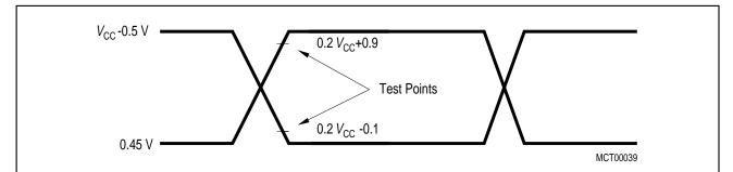
AC Inputs during testing are driven at  $V_{\rm CC}$  – 0.5 V for a logic '1' and 0.45 V for a logic '0'. Timing measurements are made at  $V_{\rm IHmin}$  for a logic '1' and  $V_{\rm ILmax}$  for a logic '0'.
