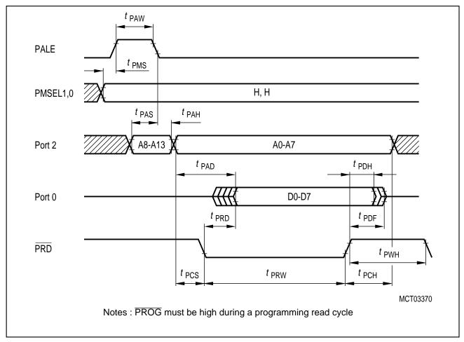
Figure 11-7 Verify Code Byte - Read Cycle Timing
