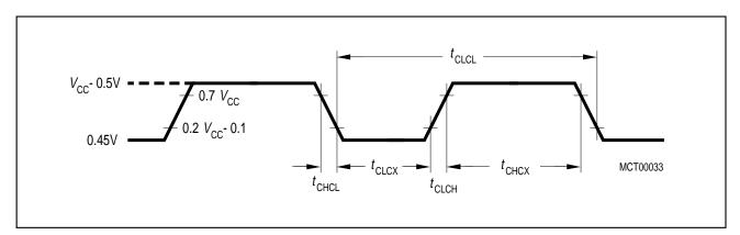
Figure 11-5 External Clock Cycle
