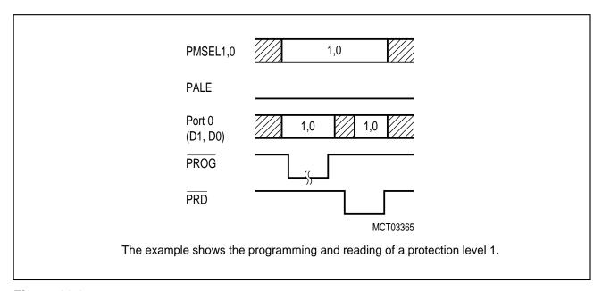
Figure 10-6 Write/Read Lock Bit Waveform
