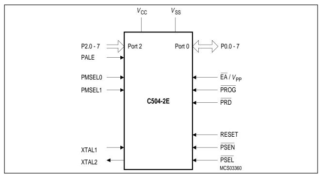
Figure 10-1 C504-2E Programming Mode Configuration
