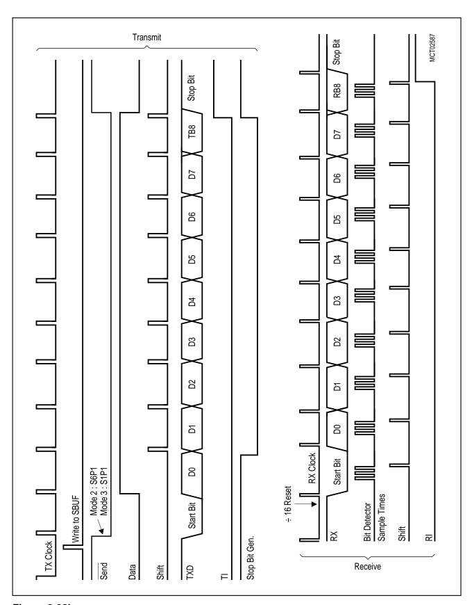
Figure 6-38b Serial Interface, Mode 2 and 3, Timing Diagram
