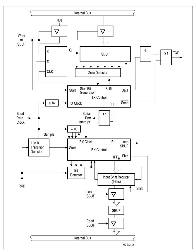
Figure 6-38a Serial Interface, Mode 2 and 3, Functional Diagram
