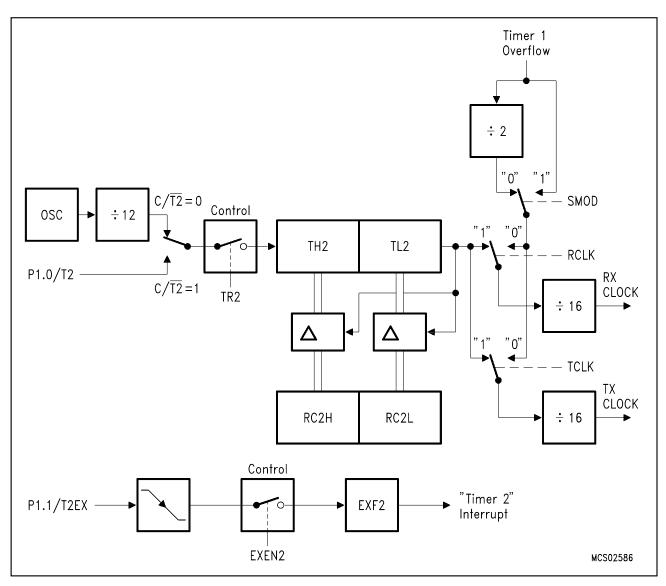
Figure 6-35 Timer 2 in Baud Rate Generator Mode
