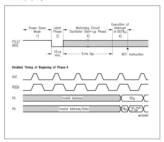
Figure 9-1 Wake-up from Power-Down Mode Procedure
