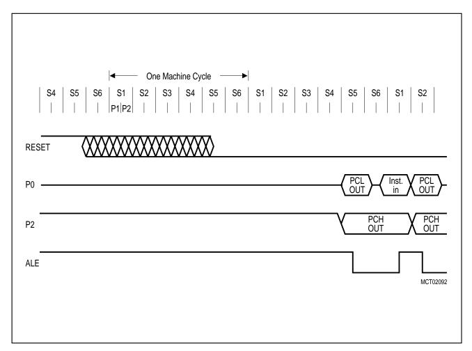
Figure 5-3 CPU Timing after Reset
