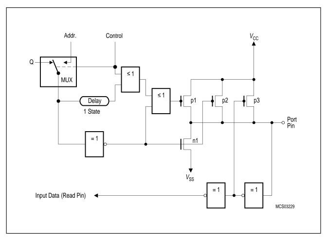
Figure 6-6 Port 2 Pull-up Arrangement
