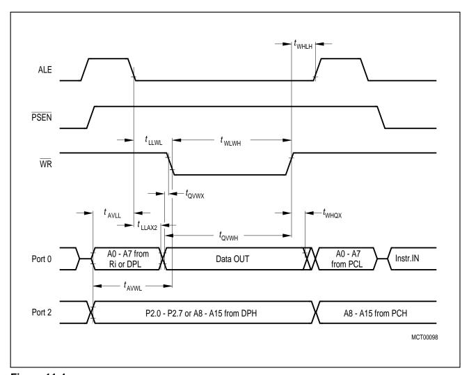
Figure 11-4 Data Memory Write Cycle
