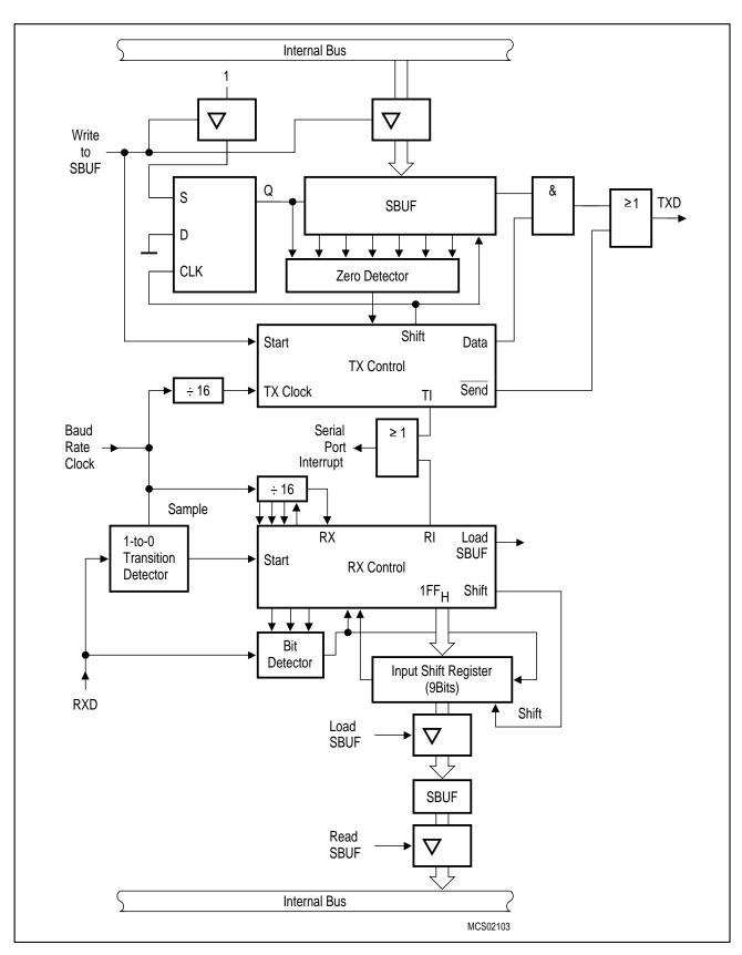
Figure 6-37a Serial Interface, Mode 1, Functional Diagram
