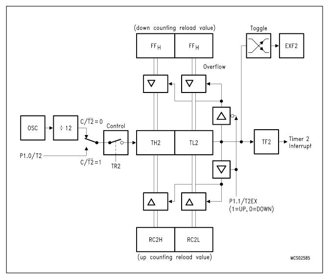
Figure 6-17 Timer 2 Auto-Reload Mode (DCEN = 1)
