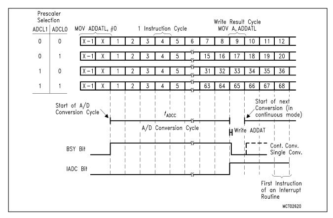
Figure 6-42 A/D Conversion Timing in Relation to Processor Cycles
