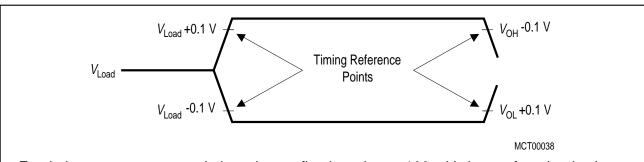
For timing purposes a port pin is no longer floating when a 100 mV change from load voltage occurs and begins to float when a 100 mV change from the loaded  $V_{\rm OH}/V_{\rm OL}$  level occurs.  $I_{\rm OL}/I_{\rm OH} \ge \pm$  20 mA
