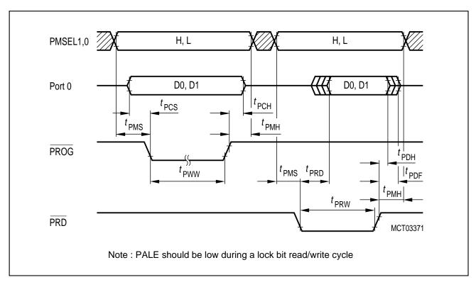
Figure 11-8 Lock Bit Access Timing
